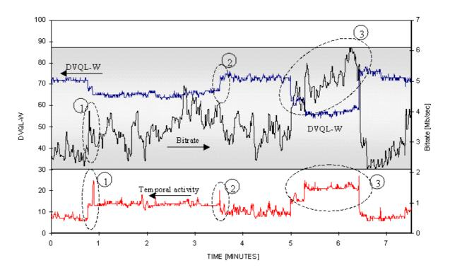
Figure 2: Measurement results for a variable bitrate programme
