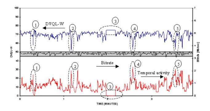
Figure 1: Measurement results for a constant bitrate programme
